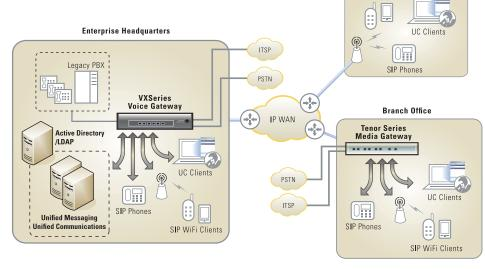
ENTERPRISE-CLASS INTEGRATION OF UNIFIED COMMUNICATIONS WITH TELECOM INFRASTRUCTURE: NET's VX Series and Tenor Series Media Gateways provide full connectivity between Unified Communications and Telecom infrastructure. NET's portfolio meets the Media Gateway requirements for UC deployments for large to small enterprises for their headquarters and branch office locations.
