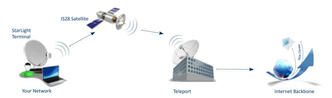
The StarLight solution is built on the world-leading Newtec Sat3play satellite access terminal with the core network implemented in Johannesburg, South Africa and which is operational on the Intelsat IS28 (NewDawn) Ku-band satellite. The IP satellite modem has embedded TCP acceleration, DNS caching and Web page pre-fetching. The use of TCP acceleration overcomes to a large extent the inherent deficiencies of TCP/IP over satellite networks.
